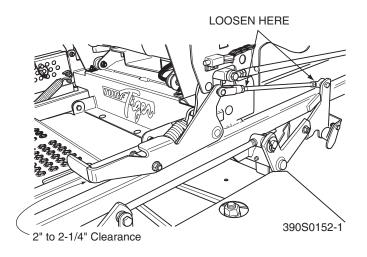
Figure 6-1. Brake Adjustment
